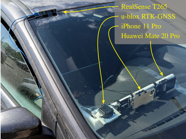
Figure 3. Car setup: GNSS is used as ground truth. Other devices record their proprietary VISLAM output (RealSense, ARKit on iOS 14.3, or ARCore 1.21) and its inputs (IMU & cameras).
