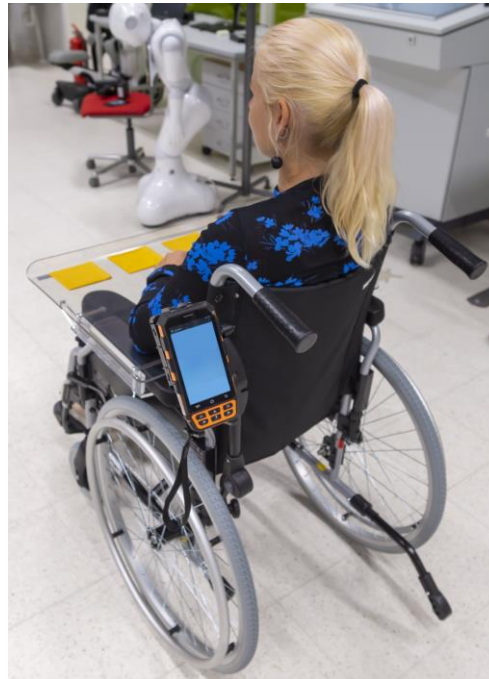
Figure 4. Measurement situation in Setup 3, RFID reader integrated in the rear left of the wheelchair.
