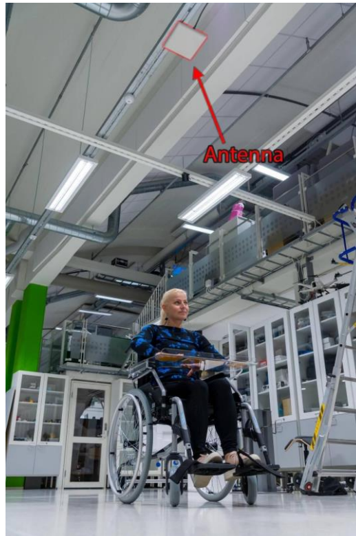
Figure 2. Measurement situation in Setup 1, reader antenna on the ceiling, wheelchair directly under the reader antenna.
