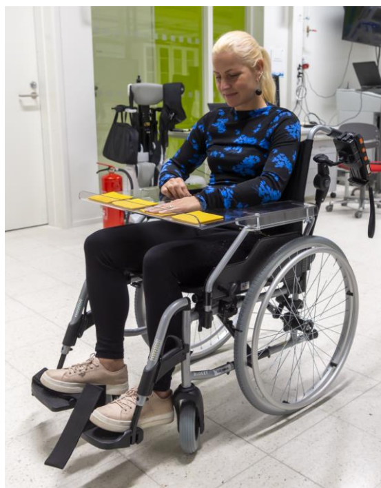
Figure 1. RFID tags are embedded inside yellow textile bags that are placed on the table tray of a wheelchair.
