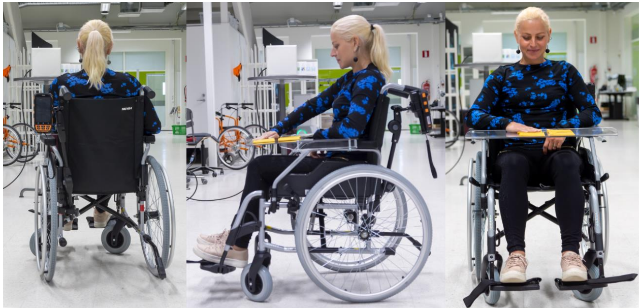
Figure 3. Measurement situations in Setup 2, reader antenna directly in front of the wheelchair (left), reader antenna directly from the wheelchair to the side (middle), and reader antenna directly behind the wheelchair.
