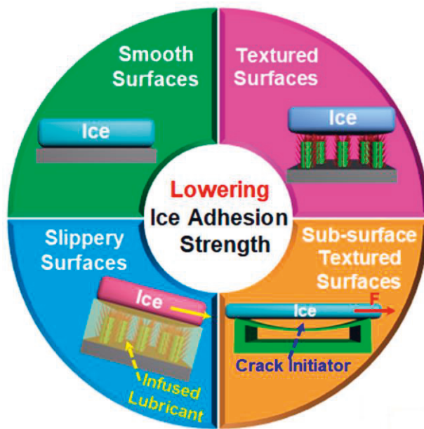
Figure 7. Strategies towards designing icephobic surfaces by lowering ice adhesion strength can be roughly divided into four types via surface properties: smooth surfaces, textured surfaces (i.e., hierarchical hydrophobic surfaces or SHSs), slippery surfaces, and sub-surface textured surfaces [112].
