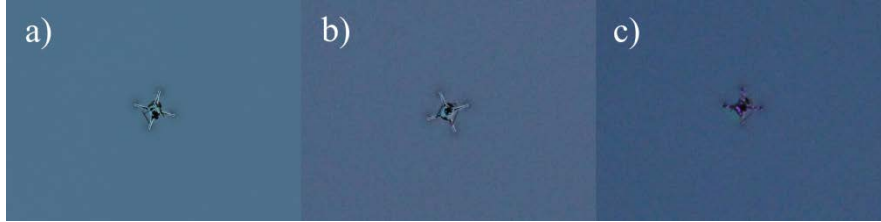
Fig. 4. The cloaked drone under extremely different lighting conditions. a) Bright sky, b) civil twilight, c) nautical twilight
