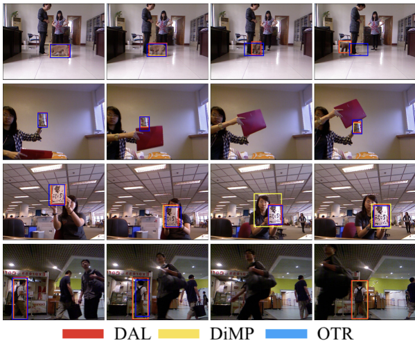
Fig. 3. Qualitative comparison of DAL, DiMP and OTR on the PTB. All trackers localize the target and give precise bounding boxes (the first two columns). With depth-modulated DCF, our tracker shows better discriminative ability when strong distractor appears (human face in the third row and human legs in the first row). Compared to DiMP and OTR, with conservative long-term tracking design, our tracker reports target disappearance more accurately.
