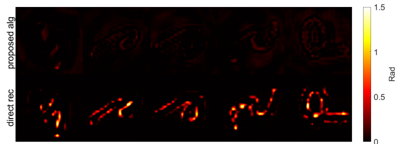
Figure 4. Errors maps of phase reconstruction provided by the proposed algorithm, top row, and direct reconstruction, bottom row, for the same objects from Fig.3.
