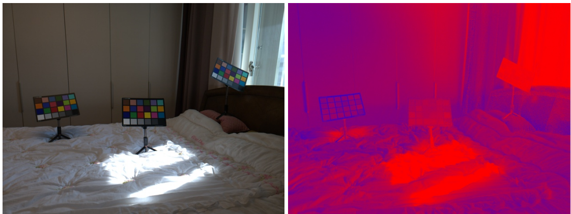
Figure 2.17. An example mixed illuminated image from the LSMI dataset with corresponding illuminant coefficient map.
