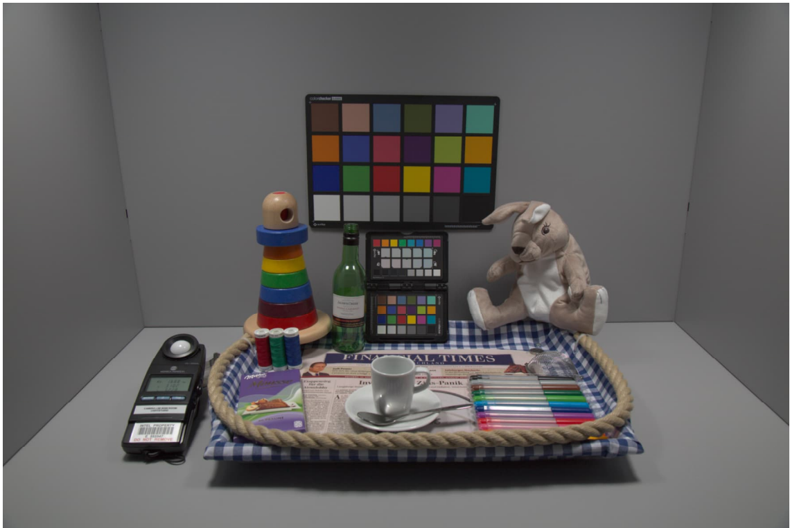
Figure 2.15. CCM applied version of the Figure 2.14 (b). Gamma is applied for visualization purposes.
