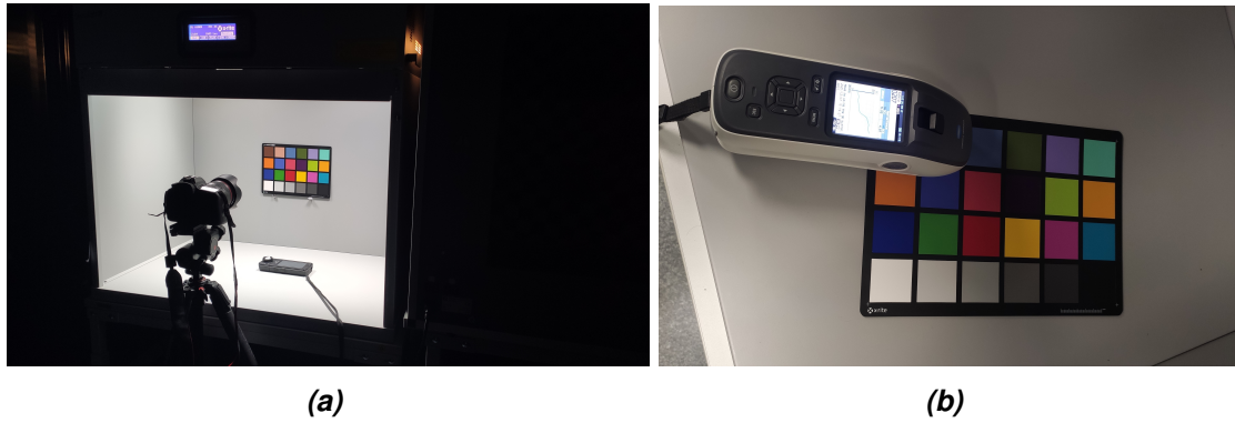
Figure 5.1. Conducted spectral measurements in the lab that is necessary for the validation experiment. On the left, the spectral power distribution measurement of 6 available light sources with Konica Minolta CL-70F is shown. On the right, spectral reflectance measurement of all patches of Color Checker Classic with Konica Minolta CM-26dG is shown.
