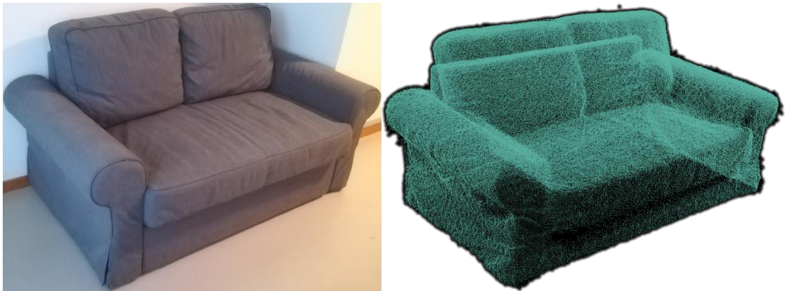
Figure 1. 3D scanned sofa and the resulting complete 3D point cloud
