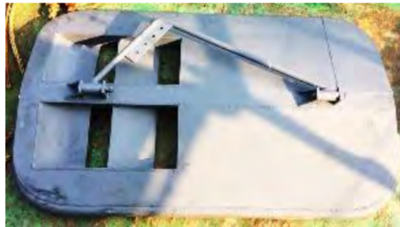
Fig.8. 1500mmx 900mm (110kg) V-form double slotted otter board
