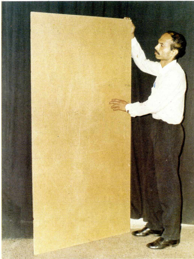
Particle Board of Size 6' x 3' x 12 mm Prepared from Cotton Plant Stalk.
