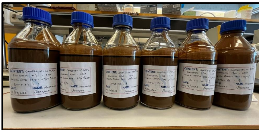
Figure 3.7 After mixing Enviromul OBM and divided into 6 bottles for storage
