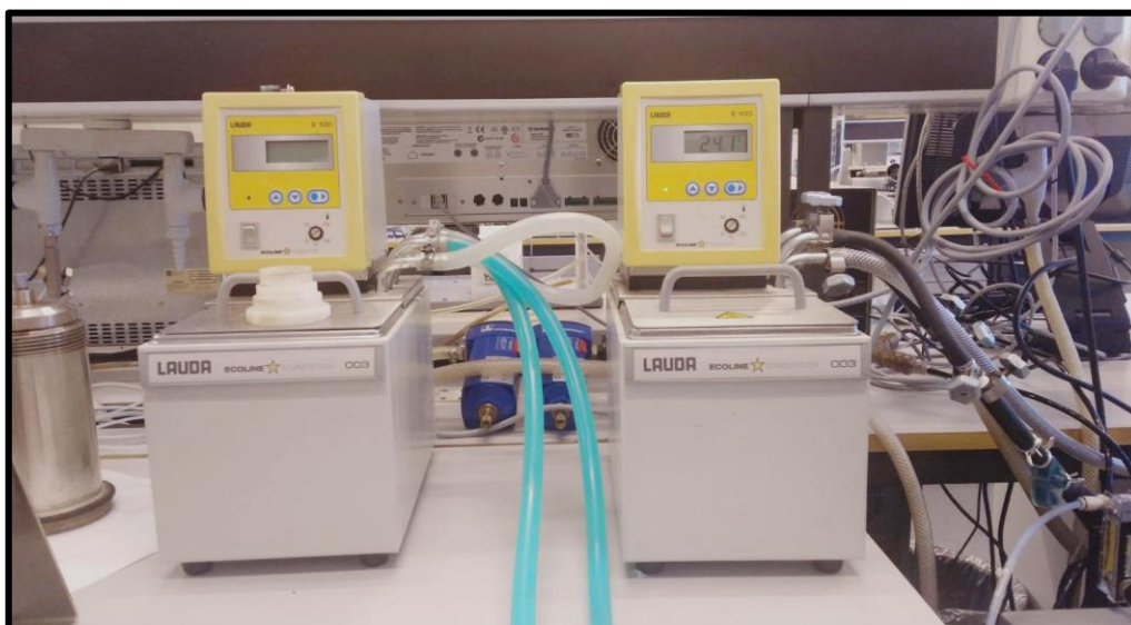
Figure 3.9 Setup showing the air supply equipment to Anton Paar MCR 302
