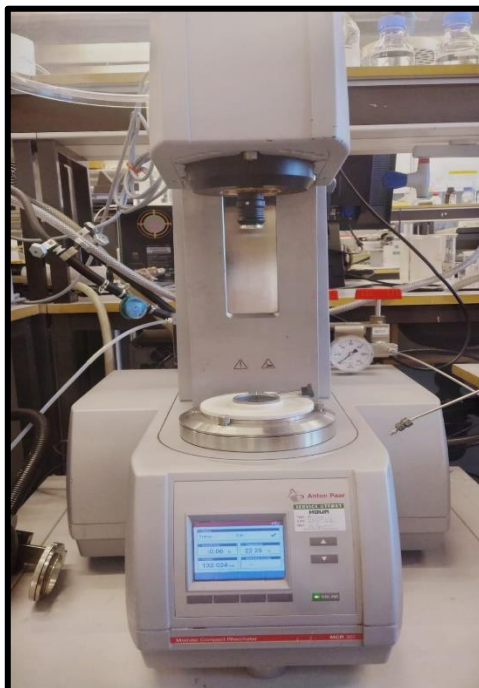
Figure 3.8 Anton Paar Modular Compact Rheometer (MCR) 302
