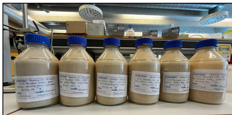
Figure 3.2 After mixing KCl Polymer WBM 1 and dividing into 6 bottles for storage
