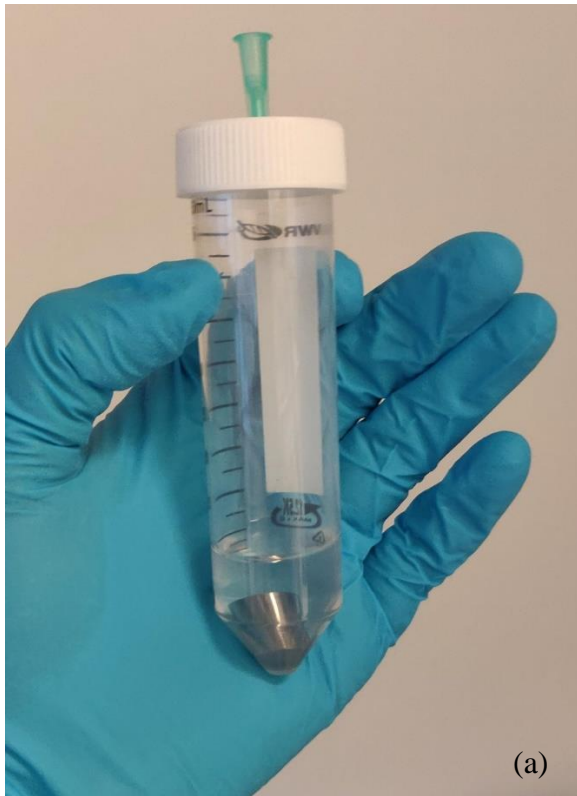
Figure 2.14 (a) Coupon submerged in acetone in a centrifuge tube. (b) Centrifuge tube containing the coupon submerged in a Branson 2510 Ultrasonic Cleaner.
