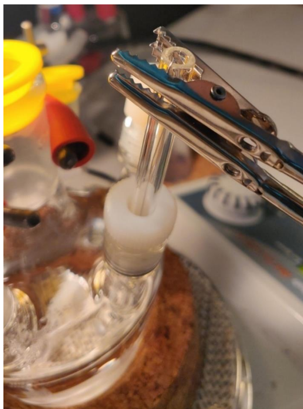
Figure 2.20 Platinum wire counter electrode, connected with clamps outside of Pyrex tube.
