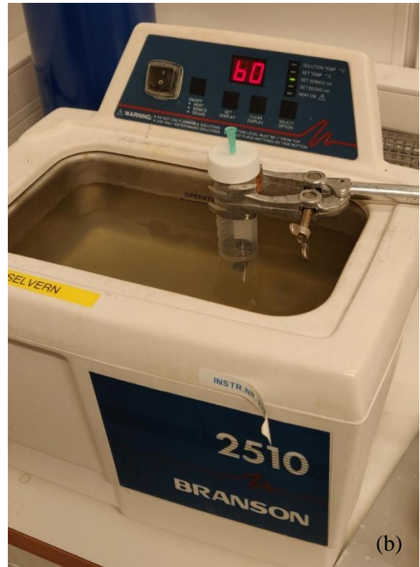
Figure 2.14 (a) Coupon submerged in acetone in a centrifuge tube. (b) Centrifuge tube containing the coupon submerged in a Branson 2510 Ultrasonic Cleaner.
