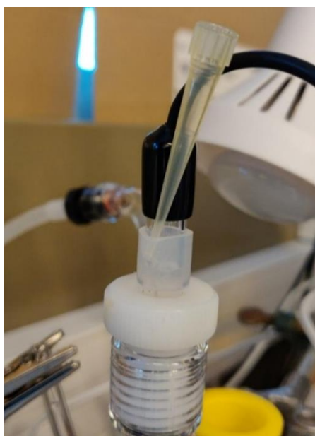
Figure 2.19 Reference electrode being ventilated by a pipette tip.
