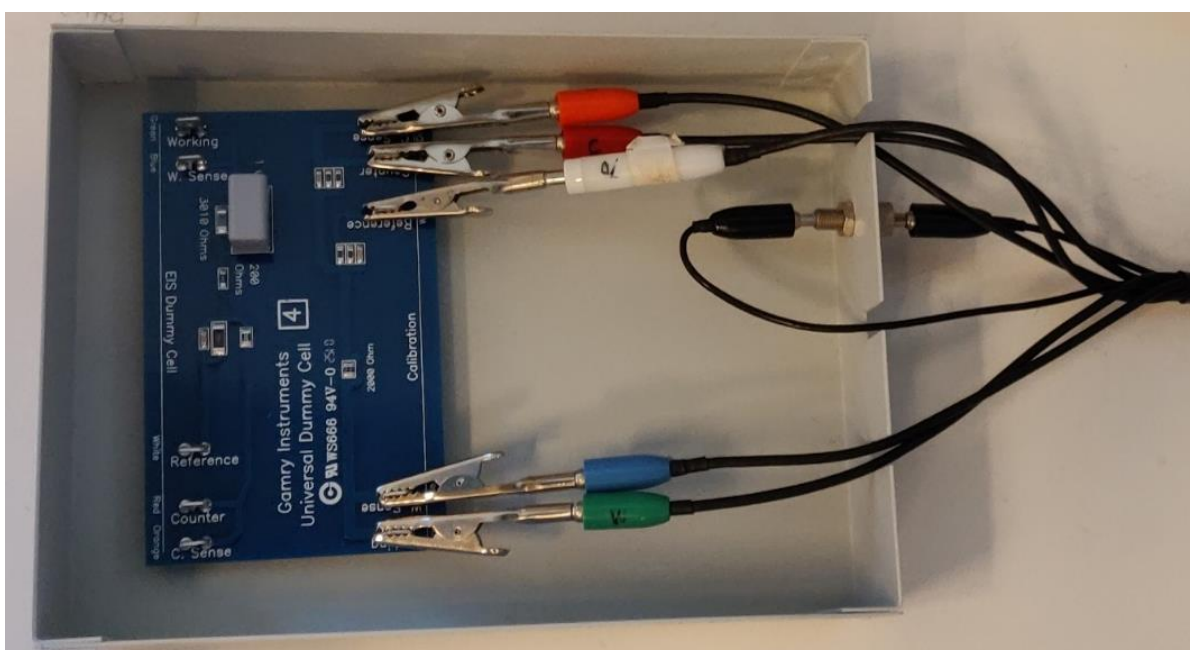
Figure 2.17 Potentiostat calibration with Gamry Instruments Universal Dummy Cell.
