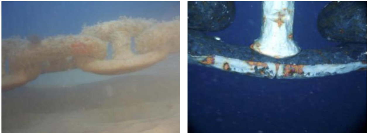
Figure 4-7: Chain Links from the Touchdown Zone, Uncleaned and Cleaned [16]
