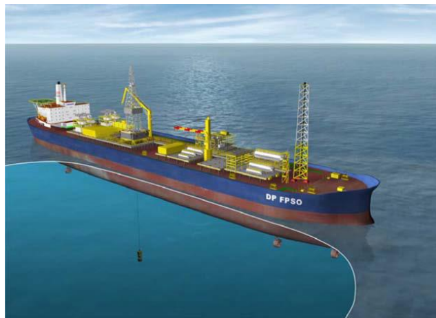
Figure 2-2: Dynamic Positioning System for an FPSO, with thrusters attached to the hull.[7]
