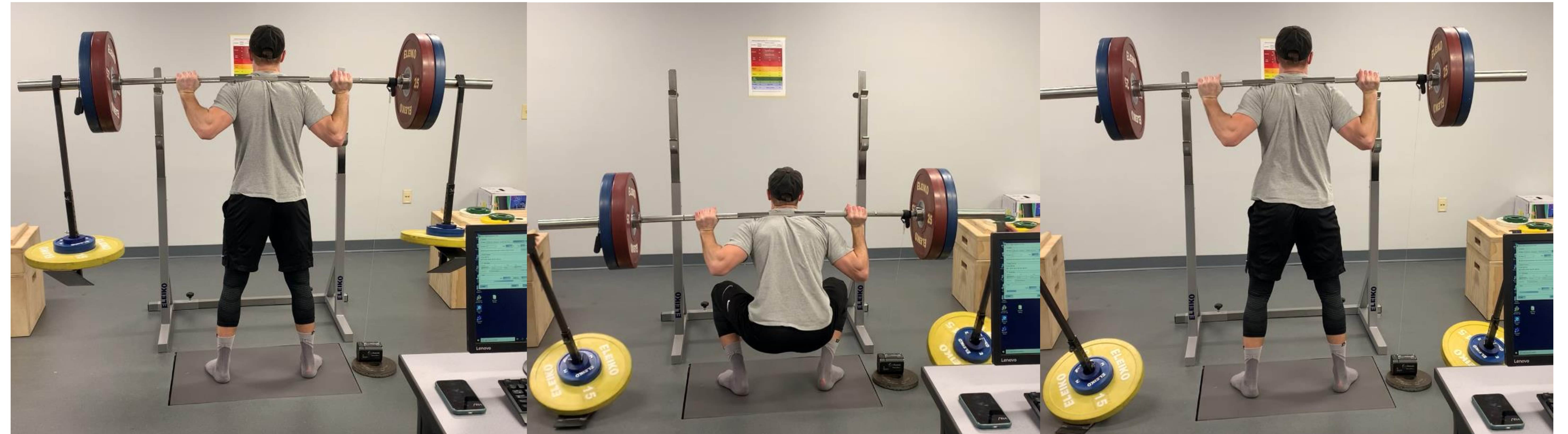
Figure 1. AEL squat sequence performed on the force platform. Subject is in the ready position (Left), end of the braking phase and start of the propulsion phase (Center), and end of the propulsion phase (Right).
