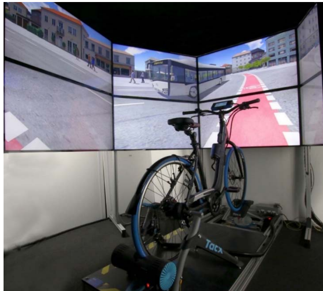
Figure 2: Bicycle simulator in front of 10 large-format displays
