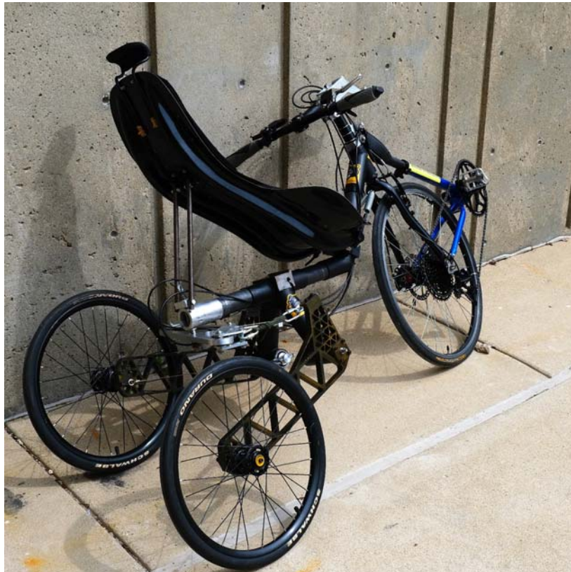
Figure 2: The working prototype in “tilting” mode leaning against a wall.
