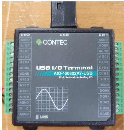
Figure 2.3: The USB I/O Terminal (right) and LEGO EV3 Brick for the motors (left)
