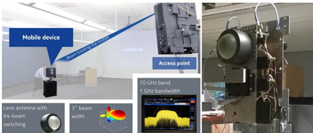
Figure 1-3 The Nokia millimeter wave (mmW) access and the backhaul demonstrators at E-band based on the beam steering lens antenna [14] .
