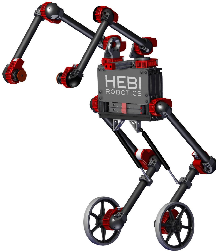
Figure A.1 A fully assembled 14 DoF Igor robot.
