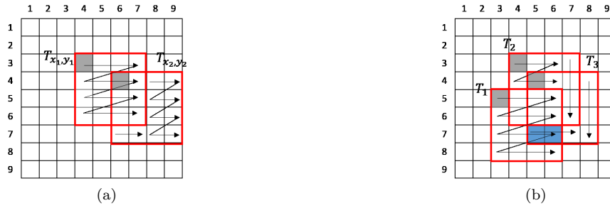
Figure 3.9: (a) Elements in the overlap region is checked only once. (b) Elements in the blue region must be checked twice.
