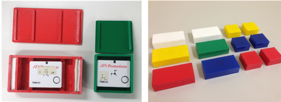
Figure 2.3: Toy blocks with the embedded Bluetooth-IMU-sensors
