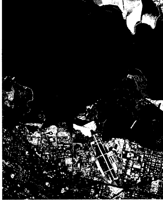
Figure 3.16 Wavelet-Based Contrast Sensitivity Fusion Results of AVIRIS Bands 30 to 40 is presented in the next section that demonstrates how well this new fusion method can fuse many bands from a hyperspectral sensor.
