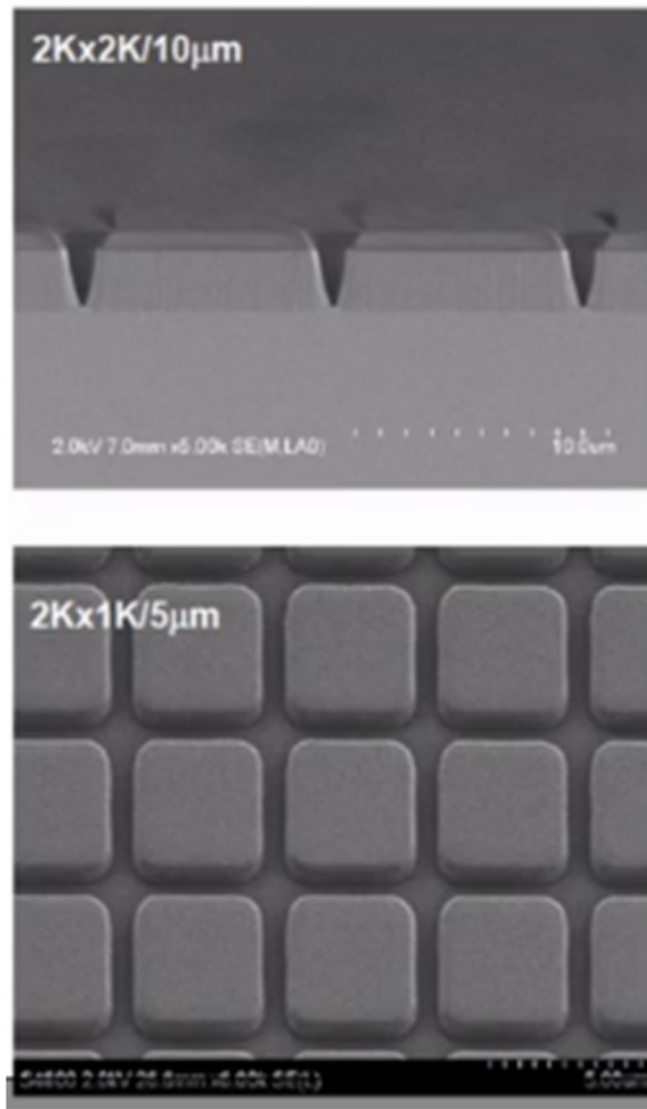
Figure 80: Scanning electron microscope images of high aspect angle pixel etches. Images taken from source with permission [61].
