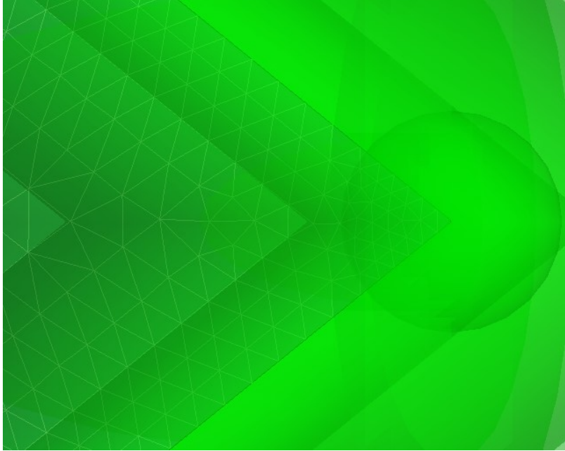
Figure 22: Mesh size at the point is a ratio to the wavelength. The point mesh is 30 points per wavelength with a of .2 wavelength radius which have 6 rows of mesh, which then flows into the variable mesh sizing from edge to smooth surface, as shown in Figure 21
