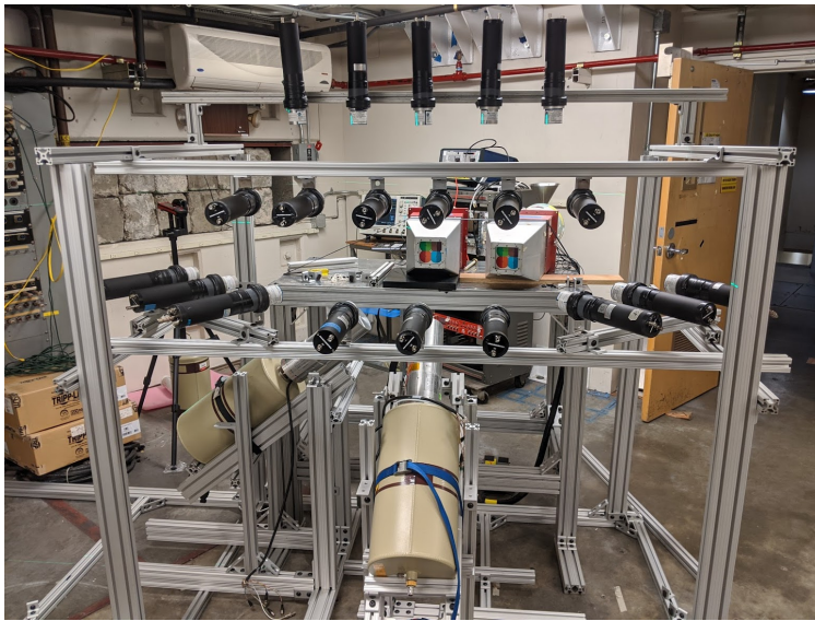
Figure 4.10. Picture of GENESIS array with HPGe clovers, HPGe Pop-Tops, and EJ-309 scintillators. The detectors were located in similar positions for this experiment.
