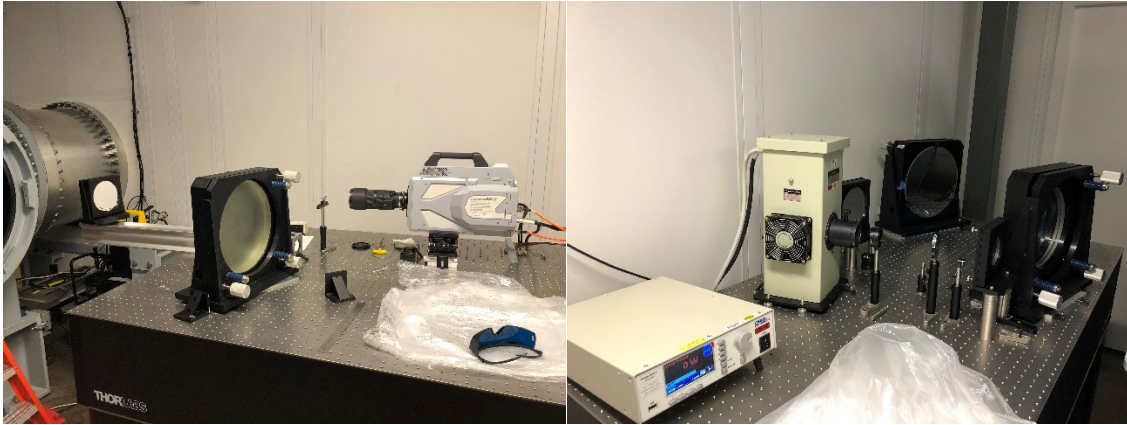
Figure 21: Physical Schlieren set-up for experiments
