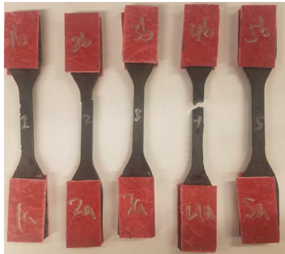
Figure 116. Epoxy-CF Specimens Batch 6 (10% reinforcement)
