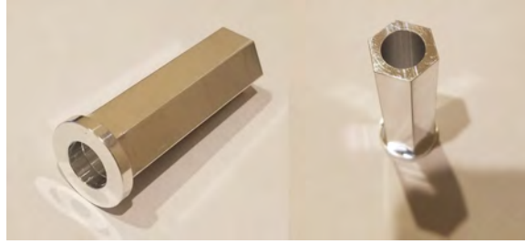
Figure 54. Aluminum Hex-Bore Sleeve Manufactured
