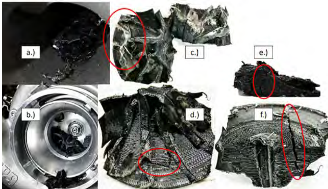
Figure 49. Post-Failure of P400 compressor, ULTEM 9085. a.) Polymer Fragments. b.) Compressor Shaft Pulled Through. c.) Two Fragments, Melted Plastic. d.) Large Fragment, Top. e.) Small Fragment. f.) Large Fragment, Bottom. Adapted from [1]
