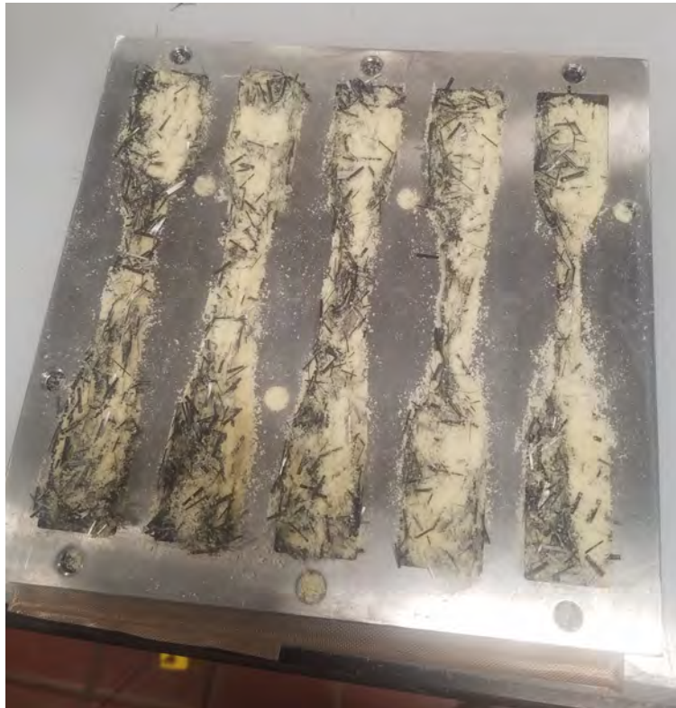
Figure 73. ULTEM 1000-carbon fiber within 3-piece Compression Mold
