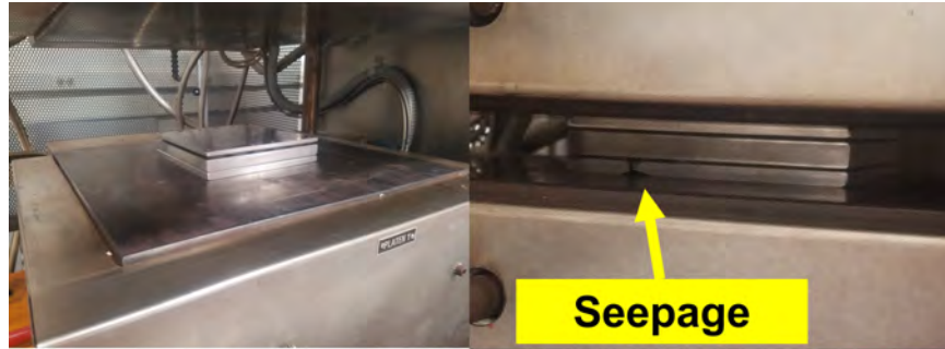
Figure 71. Batch 6 with some Seepage
