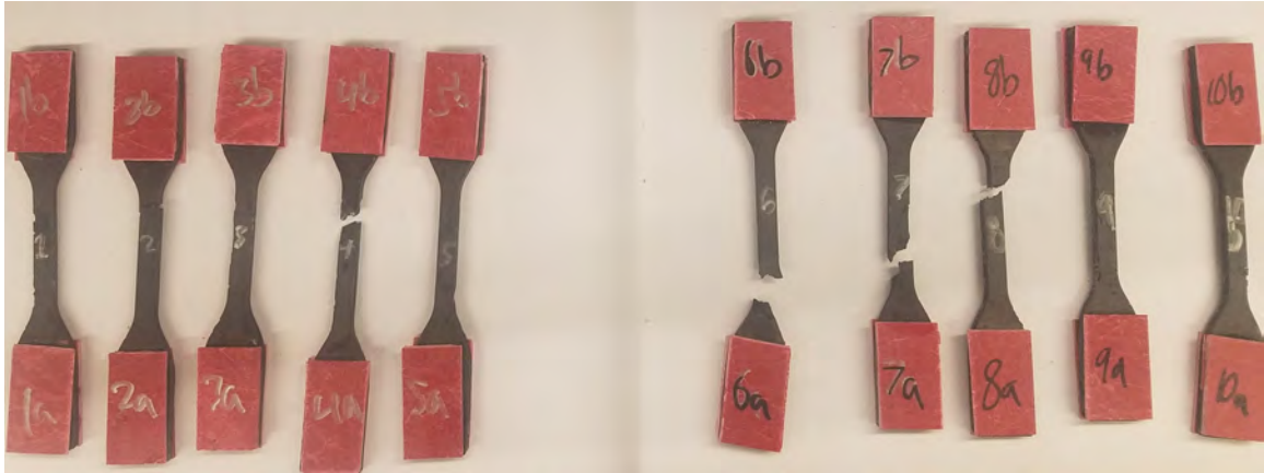
Figure 115. Epoxy-CF Specimens Batch 4 (15% reinforcement) and Batch 5 (10% reinforcement)
