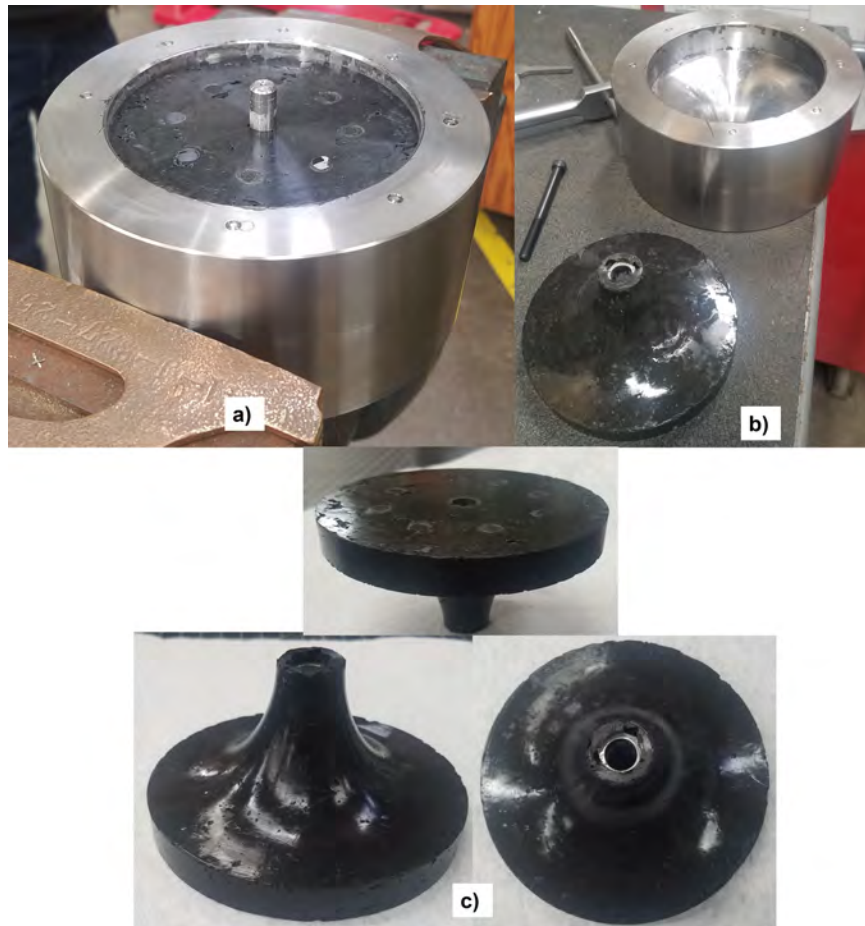
Figure 86. Compressor Hub Mold Post-Processing a) Lid up, Hub Exposed b) Hub Removed c) Hub multi-view
