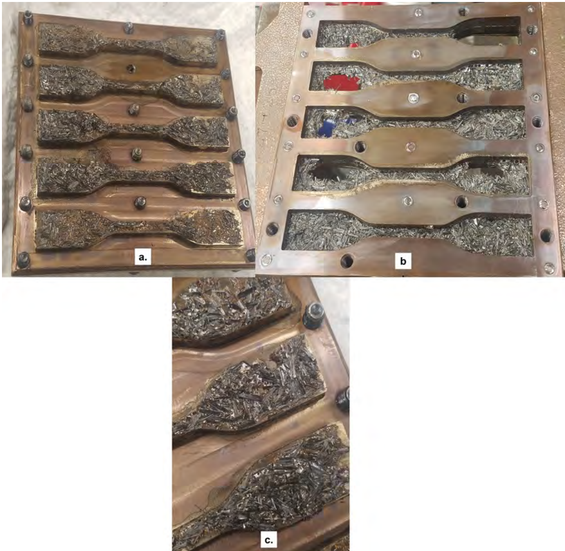
Figure 74. ULTEM 1000-carbon fiber Post Compression Specimens
