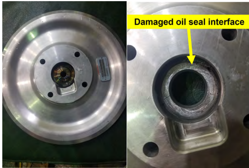
Figure 161. Damage from 2nd Turbocharger
