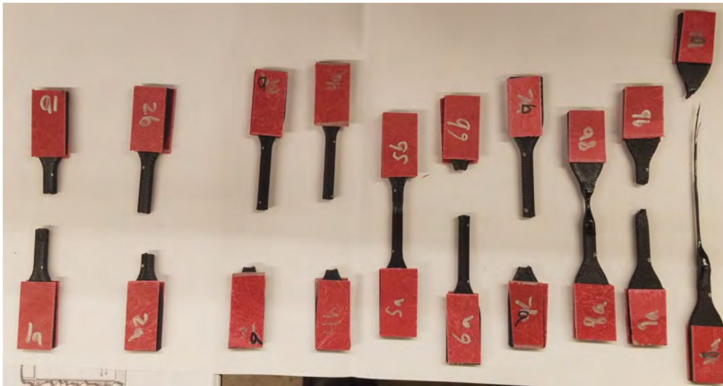
Figure 96. ULTEM 9085 specimens 1 to 10
