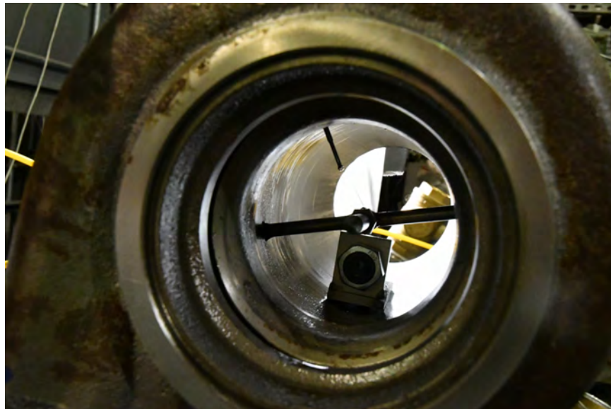
Figure 93. Turbine Axial Motion Inhibitor
