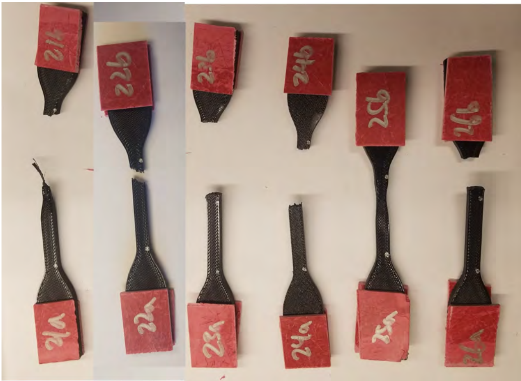
Figure 98. ULTEM 9085 specimens 21 to 26
