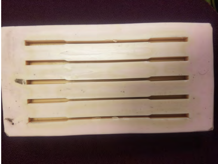
Figure 59. Specimens in Silicone Mold
