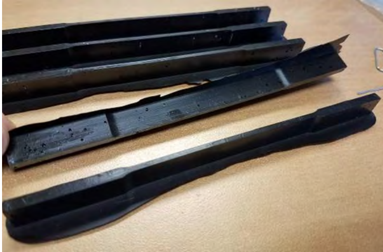
Figure 62. Batch 2: Traditional Dogbone Shape
