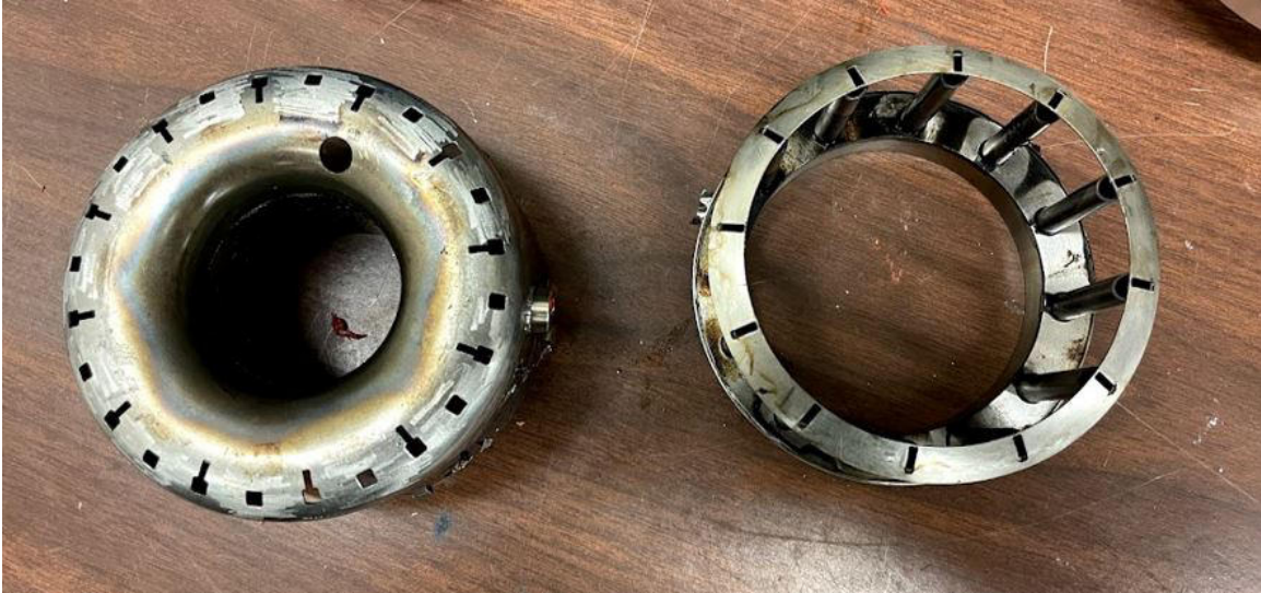
Figure 44. Top-view of the P160 compact combustor components post-machining and laser-welding
