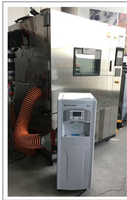
Figure 5 - Residential Device Testing Set Up [4]
