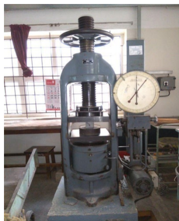
Fig. 3 - Compressive strength testing
