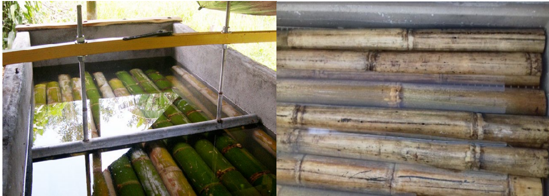
Fig. 3 - Treating bamboo by immersing in water
