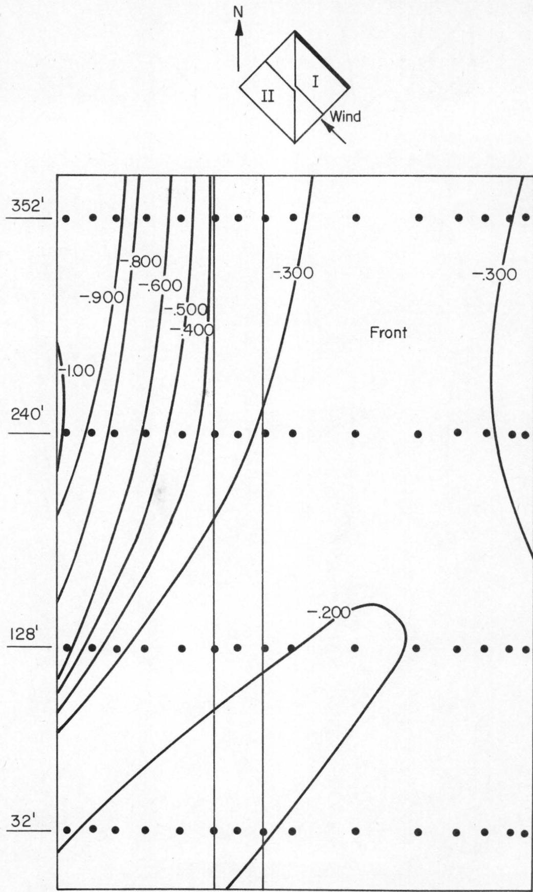
Figure 11c. Pressure contours on Building I for  $120^\circ$  azimuth wind.
