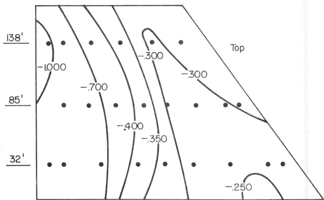
Figure 11d. Pressure contours on Building I for 120° azimuth wind.
