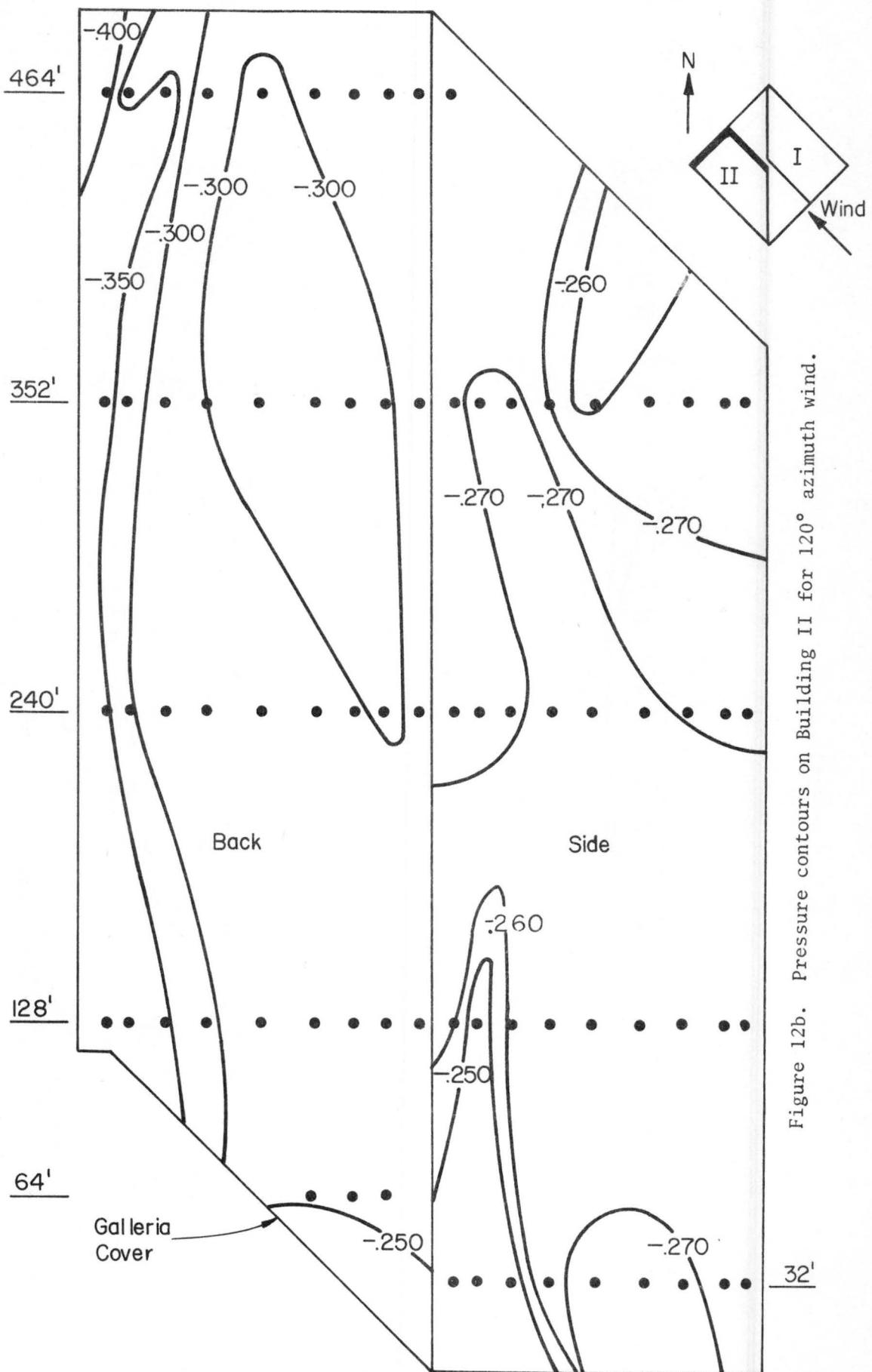
Figure 12b. Pressure contours on Building II for 120° azimuth wind.
