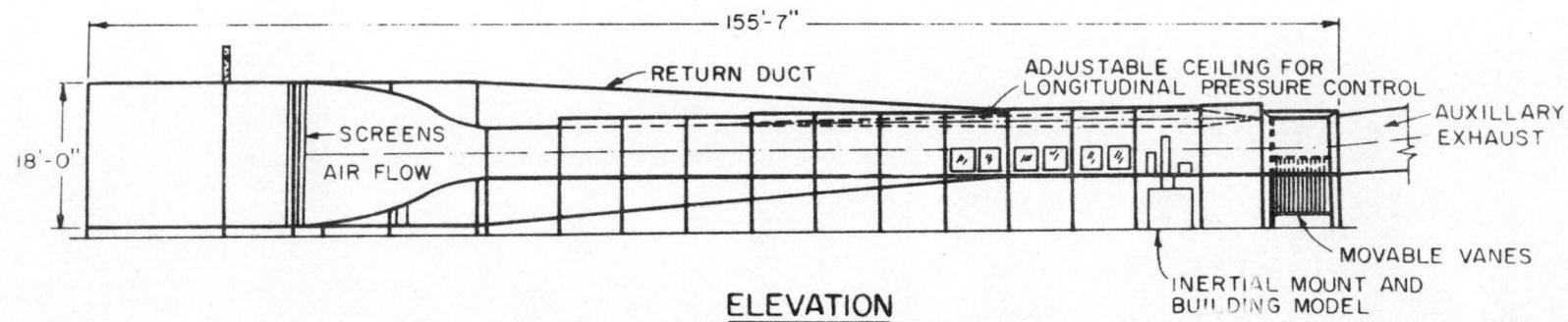
Figure 1. Plan view of meteorological wind tunnel.
