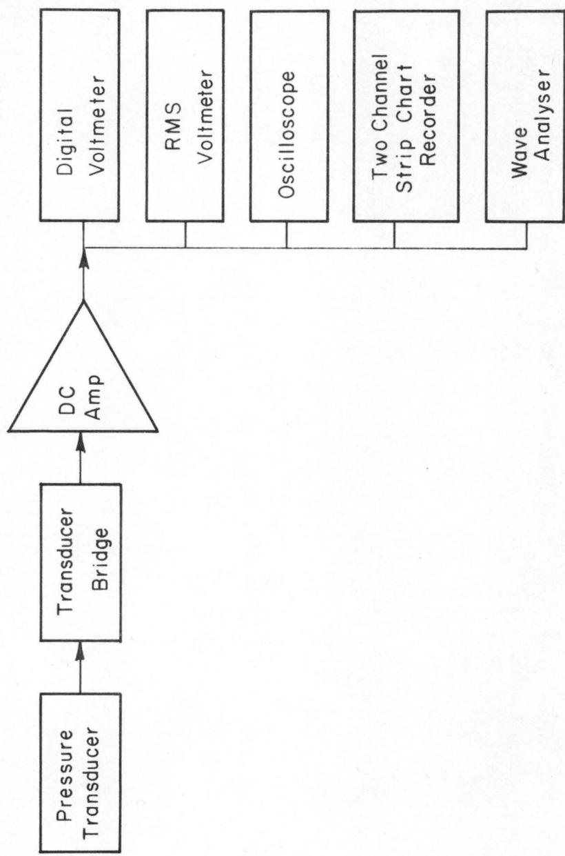
Figure 5. Block diagram of fluctuating pressure instrumentation.
