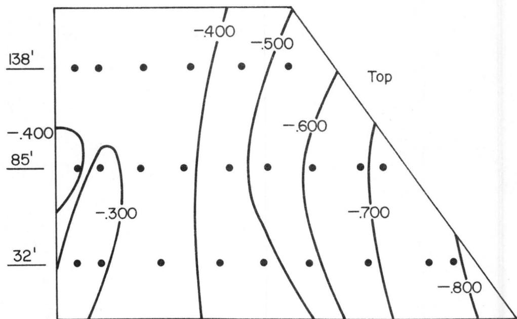
Figure 12d. Pressure contours on Building II for  $120^\circ$  azimuth wind.
