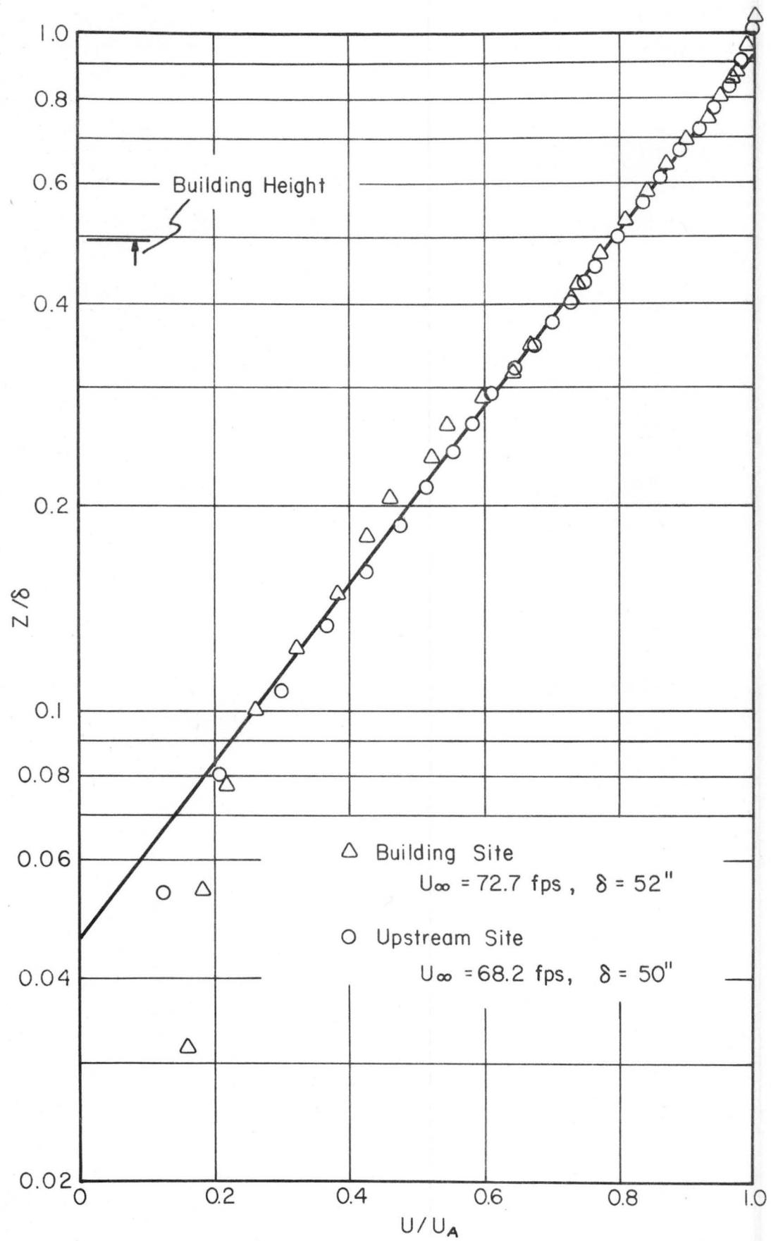
Figure 6. Mean velocity profiles.
