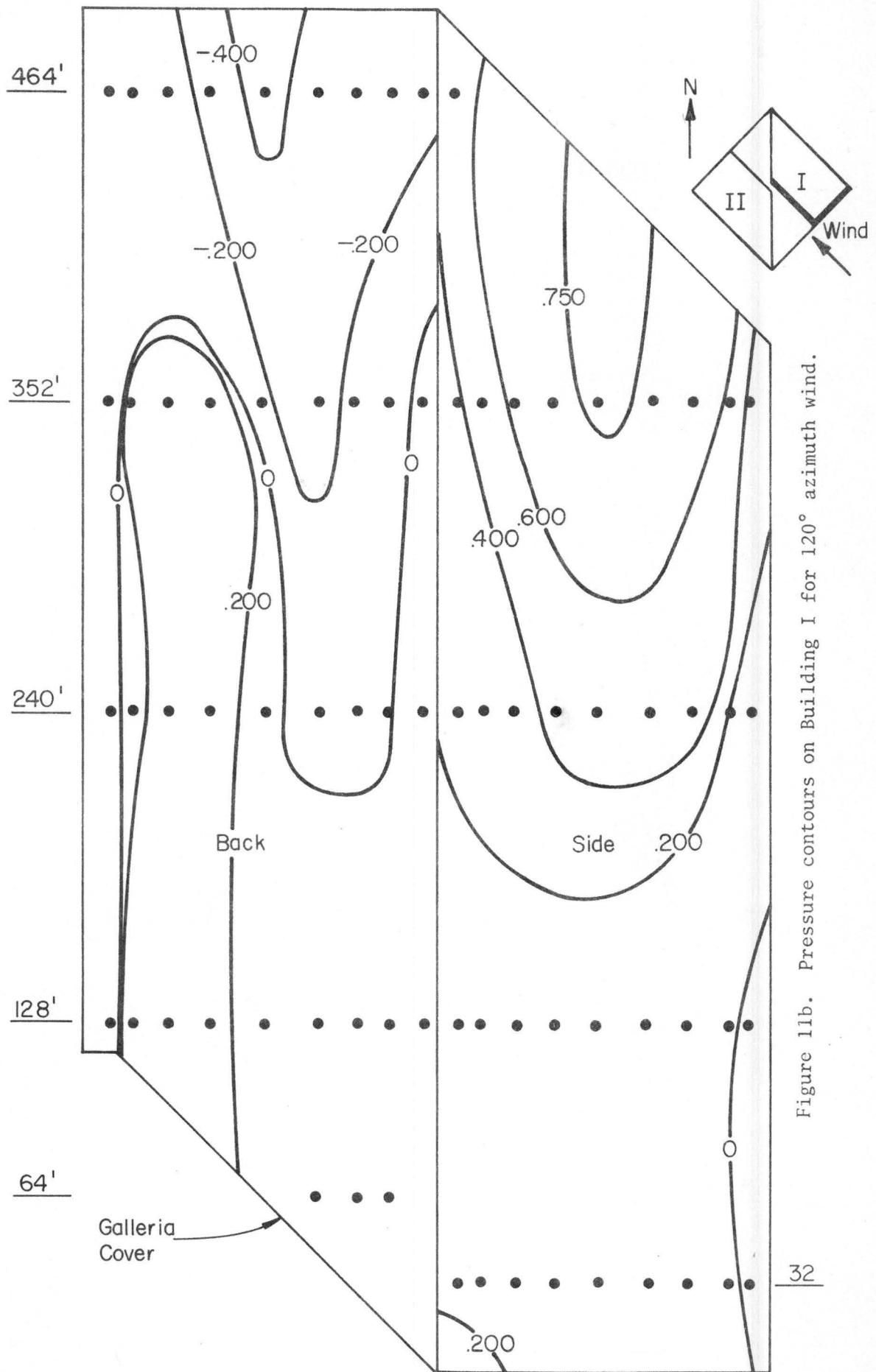
Figure 11b. Pressure contours on Building I for  $120^\circ$  azimuth wind.
