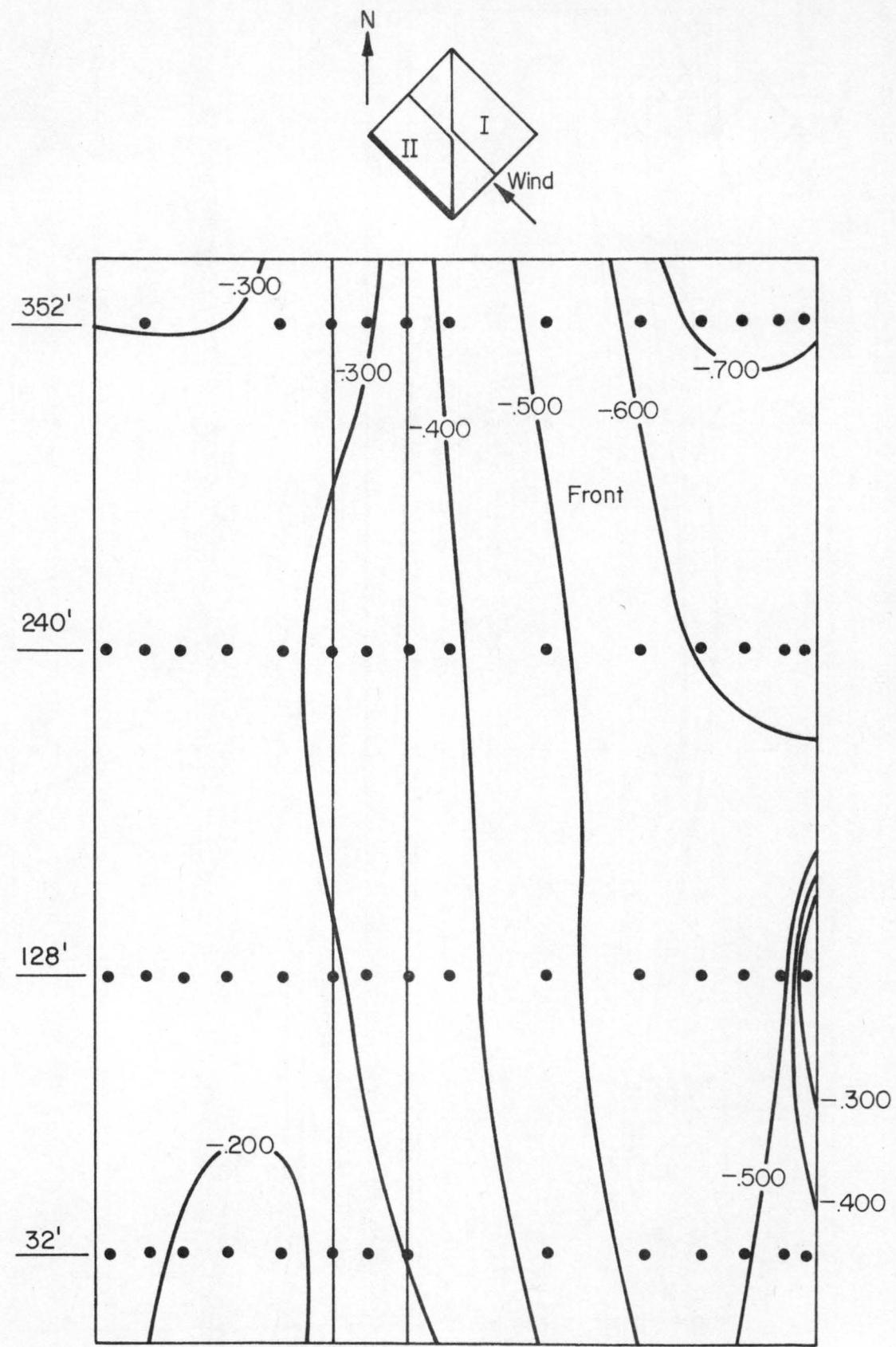
Figure 12c. Pressure contours on Building II for  $120^\circ$  azimuth wind.
