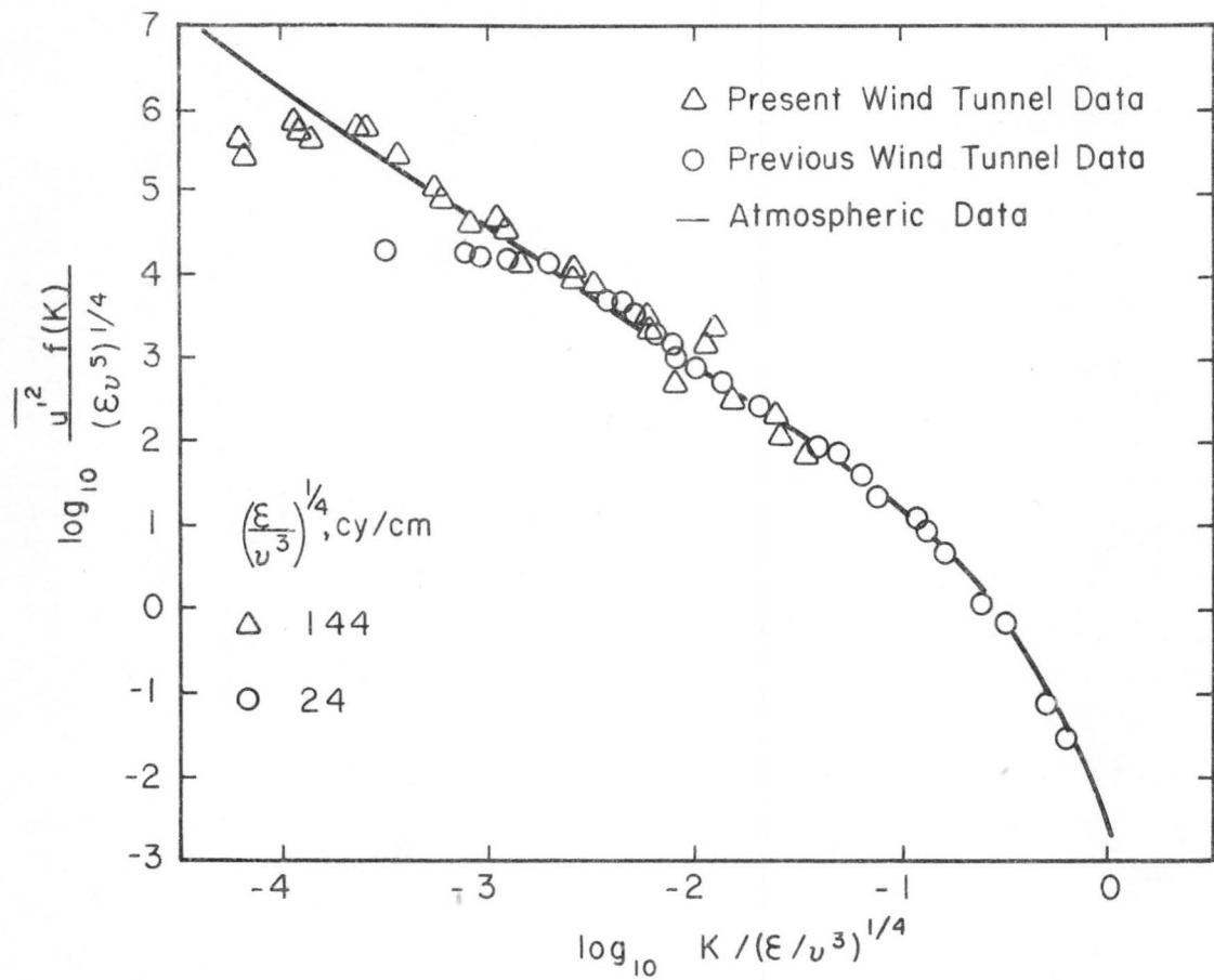
Figure 8. Comparison of velocity power spectra with previous wind-tunnel and field data.
