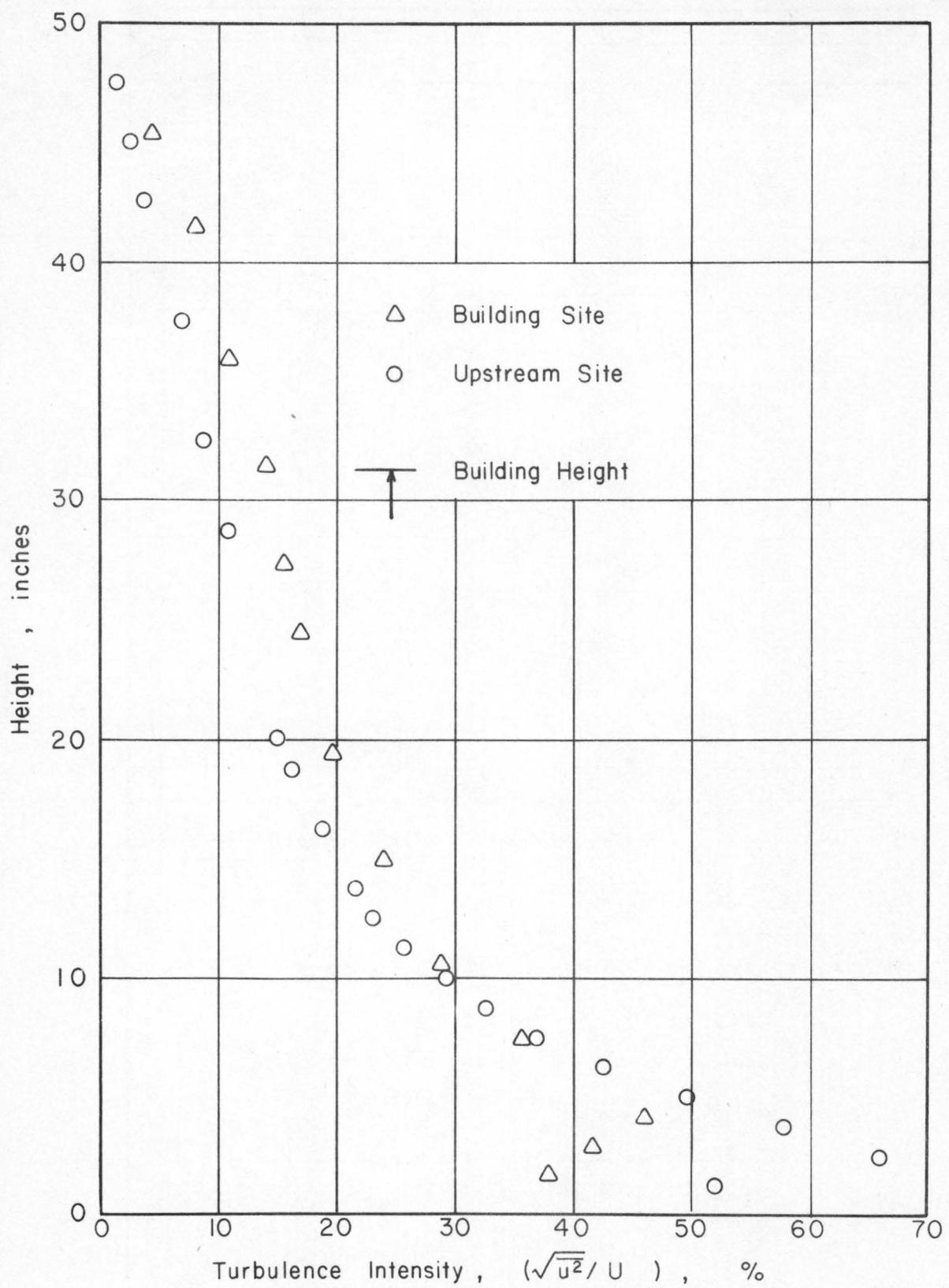
Figure 7. Turbulence intensity profiles.
