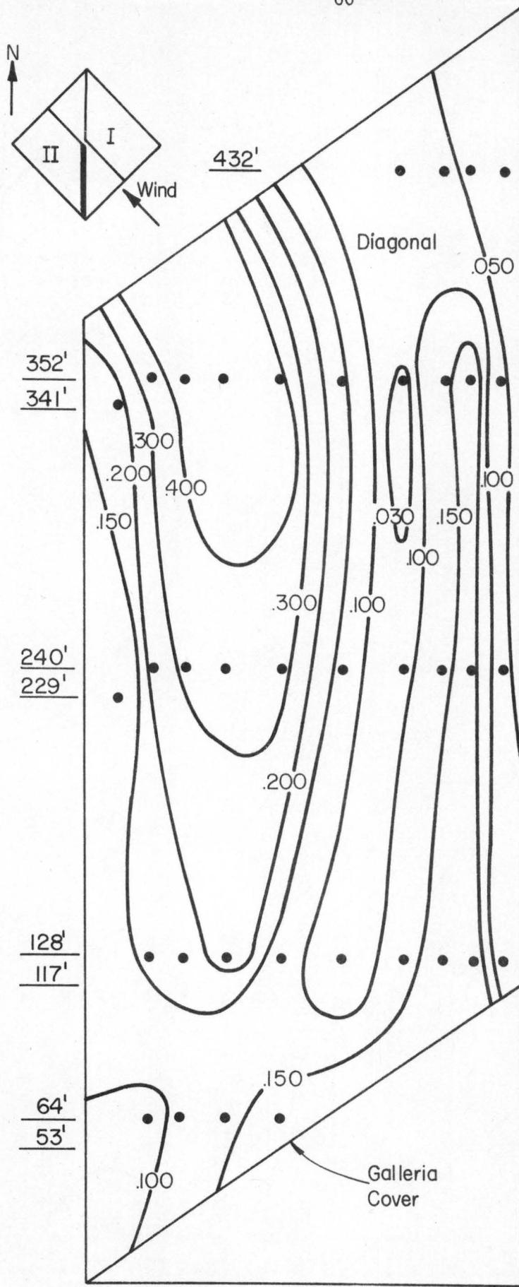
Figure 12a. Pressure contours on Building II for 120° azimuth wind.
