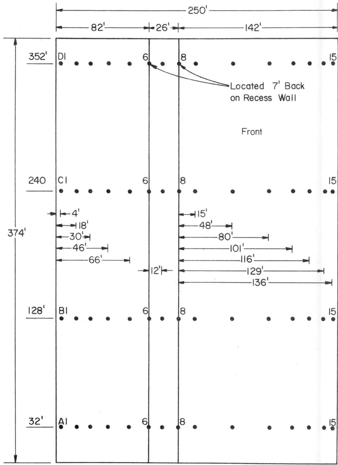
Figure 3d. Pressure tap locations and code.
