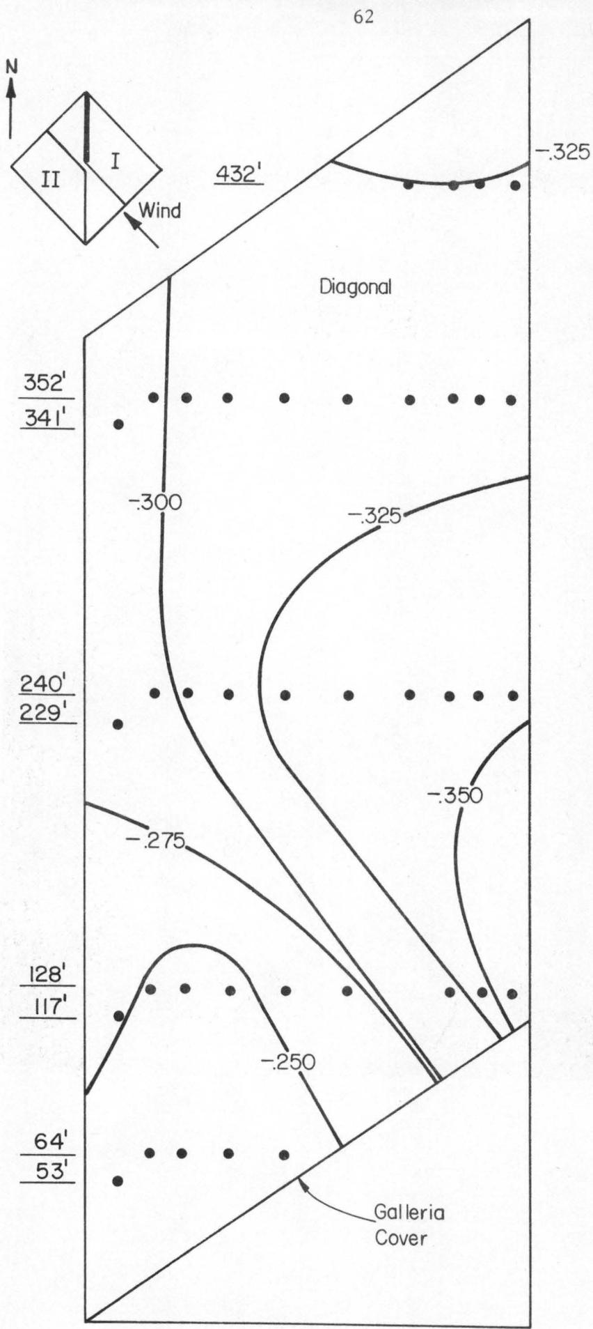
Figure 11a. Pressure contours on Building I for 120° azimuth wind.
