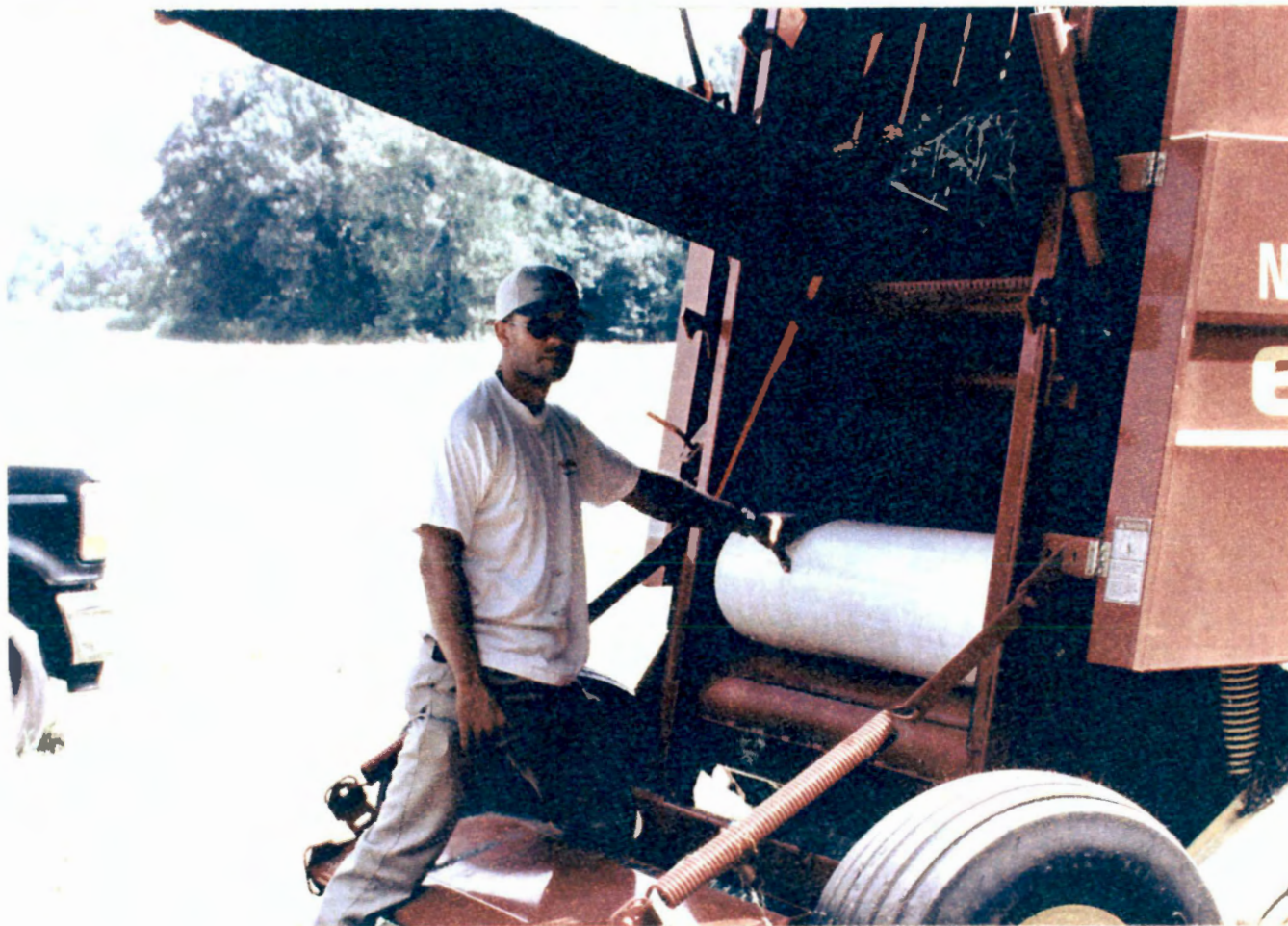
Figure 1. PVC pipe inserted into the bale chamber to form a hollow core bale
