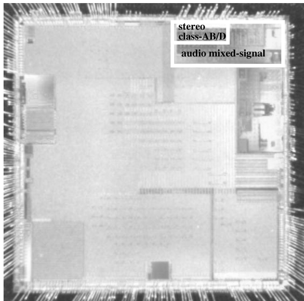
Fig. 20. Chip micrograph of full baseband including mixed-signal IPs. The audio IP is shown in the upper right corner.
