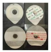
Figure 1. Ag/AgCl electrodes and its fabric composite electrode.
