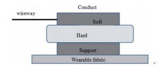
Figure 5. Structure illustration of a woven electrodes.
