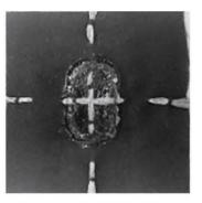
Figure 8. Embroided fabric electrodes covered with silica gel.
