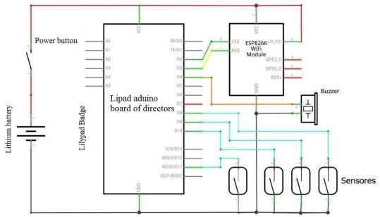
Figure 2. Schematic connection of hardware components.
