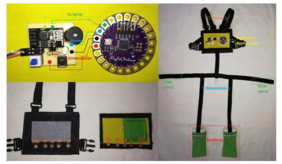
Figure 4. Integrate components into garment harness.
