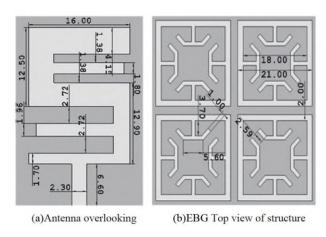
Figure 4. Antenna and EBG structure.
