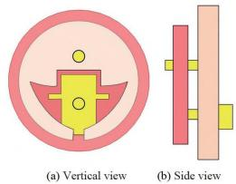
Figure 7. Structure diagram of button antenna.
