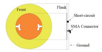
Figure 3. Wearable dual-frequency dual-mode fabric antenna.
