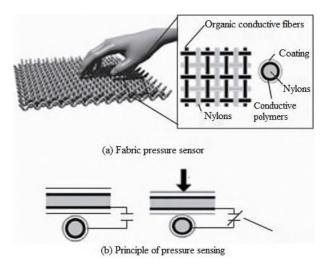
Figure 4. Schematic illustration of woven fabric pressure sensor.
