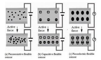
Figure 7. Schematic diagram of three flexible pressure sensors.
