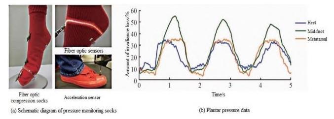
Figure 5. Pressure monitoring socks and pressure data.
