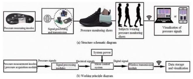
Figure 6. Structure diagram
