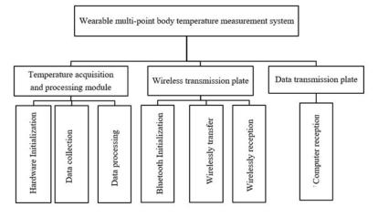
Figure 5. Block diagram of system software design.
