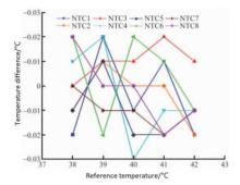
Figure 11. The measurement error of NTC thermistors.
