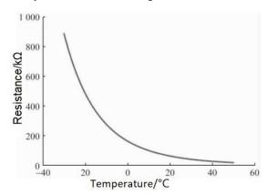
Figure 7. NTC thermistor temperature characteristic curve.
