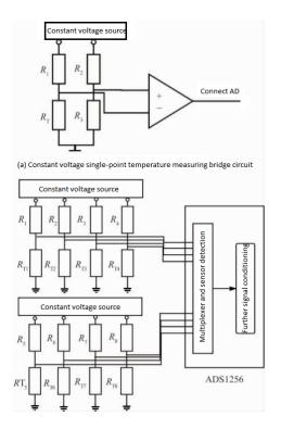
Figure 4. Single channel and multi-channel temperature measuring bridge circuit based on constant voltage.
