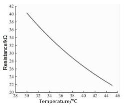
Figure 8. Stein-hart equation fitting effect diagram.
