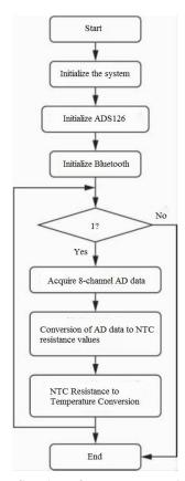
**Figure 6.** Software flowchart of temperature acquisition and processing module
