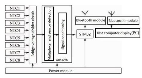
Figure 1. Block diagram of the body temperature measurement system.
