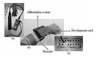
**Figure 3.** Final design of the vibrotactile handheld device. (a) Electronic control system; (b) final handheld interface mounted on an individual; (c) array of vibromotors of the device.
