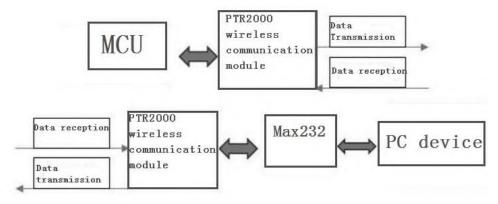
Figure 8. Working diagram of the infinite communication module.
