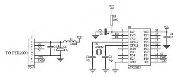
Note: (1) The first pin of AT90S2313 is the reset pin (low-level reset). (2) The second pin of AT90S2313 is the serial input pin; the third pin of AT90S2313 is the serial output pin. (3) PWR, TXEN, CS of the wireless module can be connected to any I/O of AT90S2313 for control. (4) It is recommended to use tantalum capacitors for C6.
