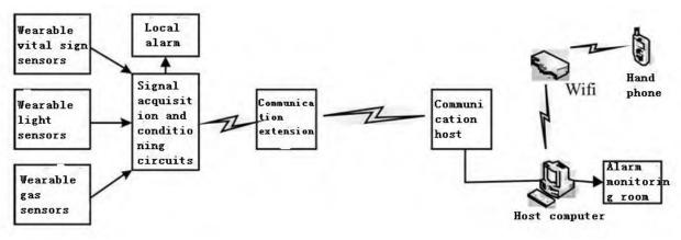
Figure 1. General diagram of system structure.
