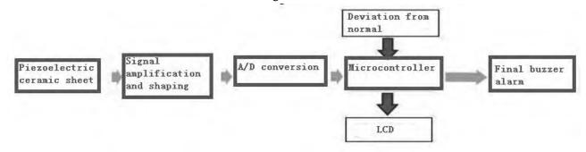
Figure 3. Structure diagram of the respiratory monitoring module.
