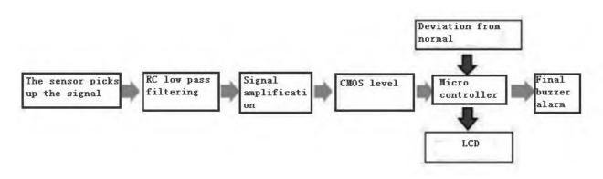
Figure 4. Structure diagram of the pulse monitoring module.
