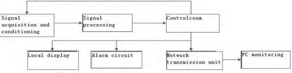
Figure 2. Working diagram of gas concentration detection module.
