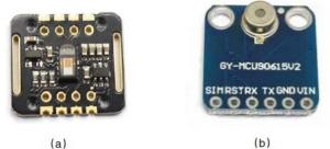
Figure 3. Blood oxygen heart rate acquisition module, temperature measurement module.
