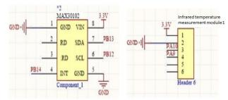
Figure 4. Acquisition module circuit connection.
