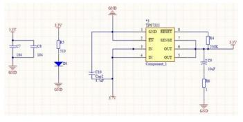
Figure 6. Power circuit.
