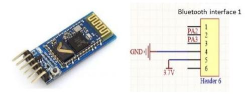
Figure 5. Bluetooth module and circuit connection.
