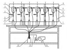
Sampling platform; 2. Outdoor rainwater collection and introduction conduit; 3. Rainwater inlet valve; 4.
