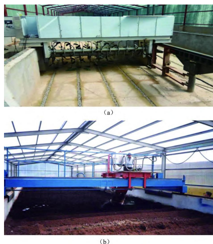
Figure 8. Intelligent trough manure treatment equipment
