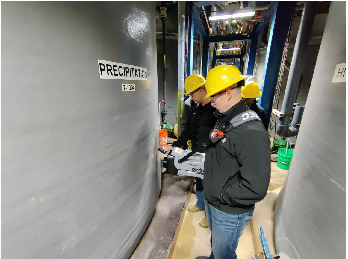
Figure 2. Maj. Jonathan W. Schwarz and Capt. Derek D. Whipkey take spectroscopy of U3O8 precipitation tanks at Nichols Ranch in-situ recovery plant near Casper, Wyoming. During Operation Pay Dirt, the Aberdeen Proving Ground, Maryland-based Nuclear Disablement Team 1 trained at the White Mesa uranium mill in Utah and the Nichols Ranch in-situ recovery mine and plant north of Casper, Wyoming, April 4 - 8. U.S. Army photo by Maj. Mark S. Quint.
