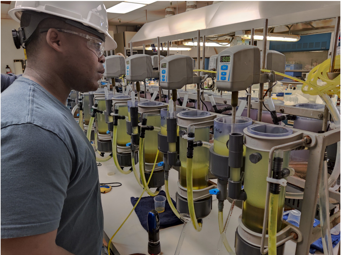
Figure 4. Sgt. Joshua M. Kamami examines a bank of mixer settlers during rare earth element recovery operations at White Mesa Uranium Mill near Casper, Wyoming. During Operation Pay Dirt, the Aberdeen Proving Ground, Maryland-based Nuclear Disablement Team 1 trained at the White Mesa uranium mill in Utah and the Nichols Ranch in-situ recovery mine and plant north of Casper, Wyoming, April 4 - 8. U.S. Army photo by Maj. Mark S. Quint.
