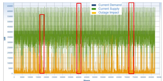
FIGURE 4: 100-YEAR SIMULATION OF ENERGY SUPPLY AND DEMAND AT FORT BENNING, INCLUDING BLACK SWAN OUTAGE EVENTS.
