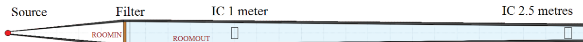
Figure 1 – Graphical representation of the Monte Carlo model for the HVL calculation. IC 1 m and IC 2.5 m correspond to the location of the active volume of the ionization chambers at a distance of 1 m and 2.5 m from the source (created by using FLAIR program [5])
