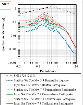
Fig. 6. Result of spectral acceleration in the study area.
