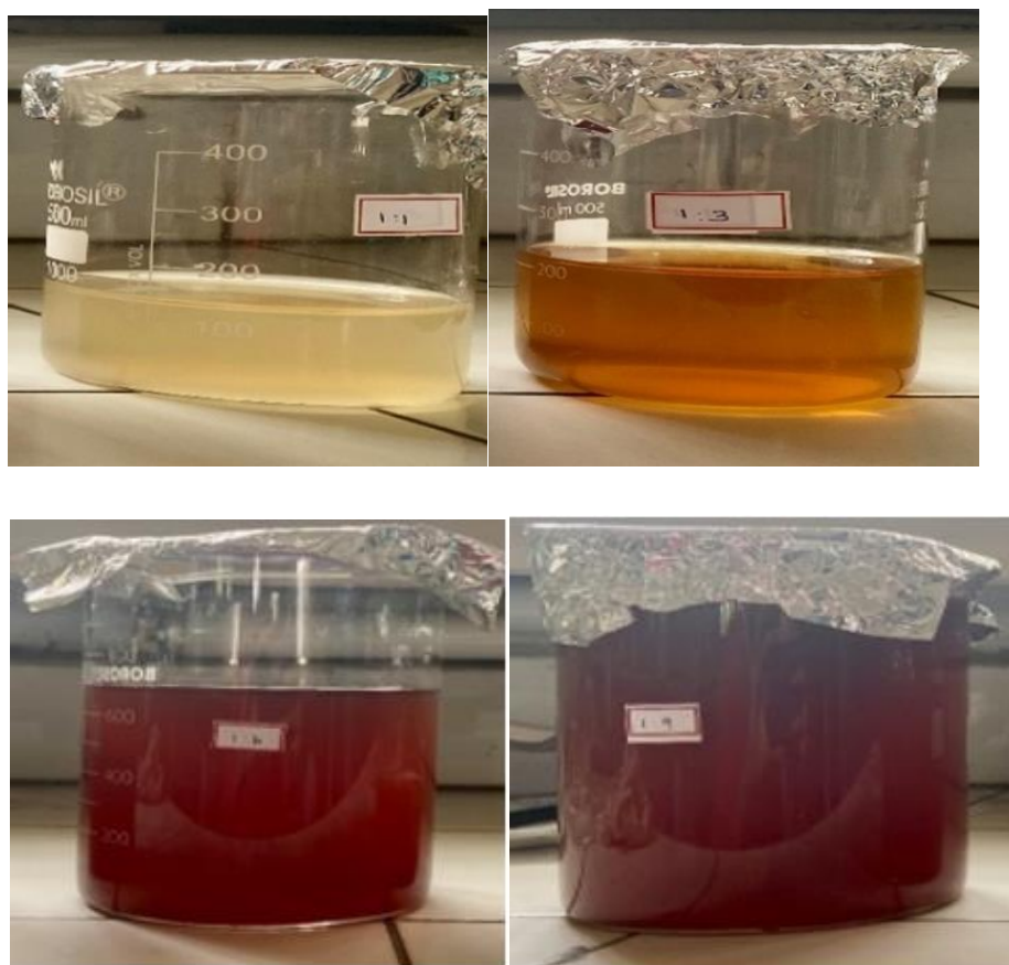
Figure no.6: Colour change for the selection of appropriate ratio after the development of silver nanoparticles.
