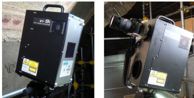
Figure 5. Left: Konica Minolta Vivid 9i. Right: Olympus E-510 rigidly connected to the scanner.
