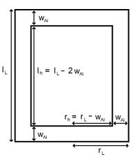
Figure 1: A cross-sectional schematic of the rocket, outlining the definitions of  $r_h$  and  $l_h$ .
